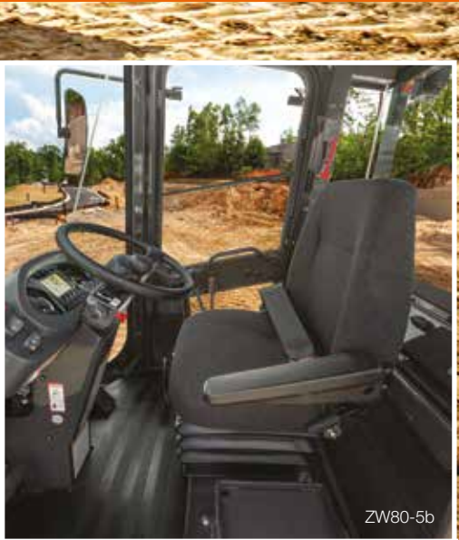
A standard long-stroke suspension seat absorbs shock and vibration (ZW80-5b).
