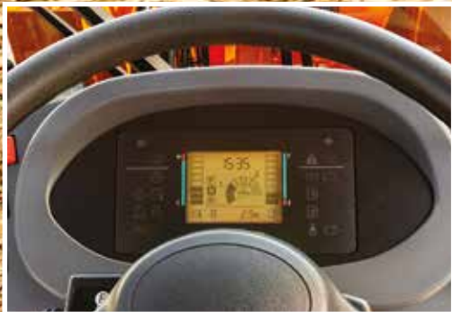
Easy to read monitor provides operating data at a glance (ZW50-5b)
