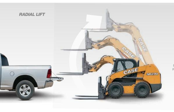
Radial-lift machines are engineered for digging, prying and pushing. The angle of the arm ties directly into the chassis for superior strength when digging and pushing. It also provides maximum reach at the operator's head height, making it perfect for loading and unloading pallets from trucks.
