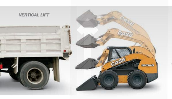
Vertical-lift machines are engineered for lift-and-carry and truck-loading jobs. The geometry of the dual arm allows the load to rise directly up, providing maximum reach at full height.
